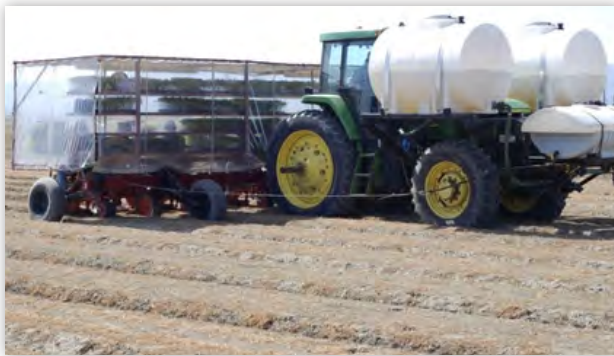
Figure 11. A conventional five-row tomato Checci Magli transplanter used to establish tomato seedlings in cover crop residues at Sano Farms, 2009.
