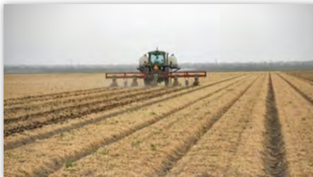
Figure 9. A ground-driven strip tiller used to prepare bed centers prior to tomato transplanting, Sano Farms, 2009.
